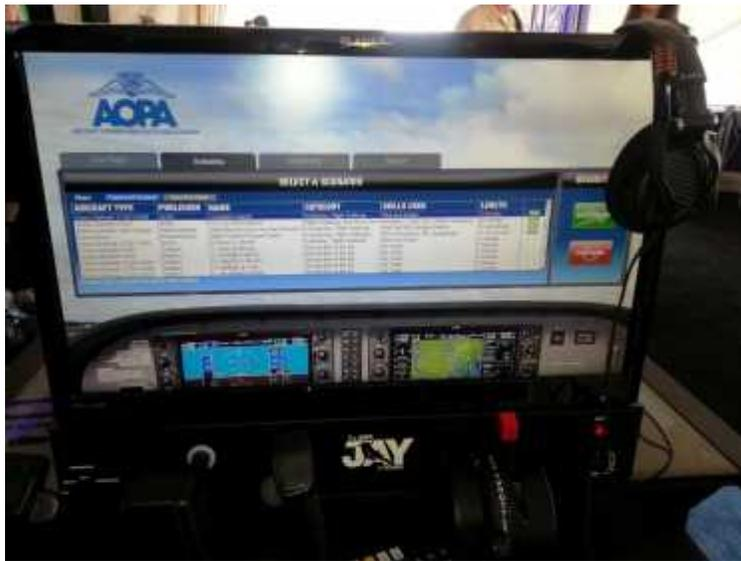
Simple Single Screen unit or multi screen unit with current Garmin electronics installed
